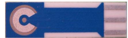
Electrochemical sensor with integrated resistors
