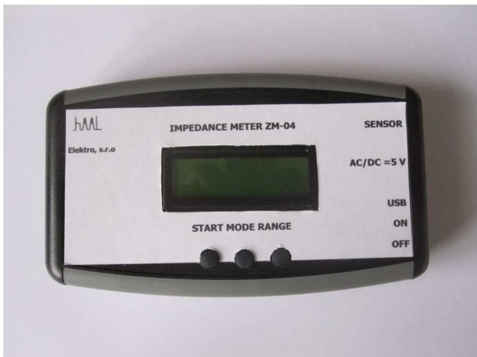
Fig. 2. Automatic impedance spectrometer HAAL Elektro ZM-04, that has been used for electrochemical cell impedance characteristic.
