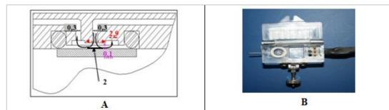
Fig. 1. A: Arrangement of flow cell FC2 wall jet. (Cell dimensions are given in millimeters.) B. FC2 wall-jet photo.
