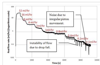
Fig. 3. Real flow rate in time PUMP AVM Technic I.
