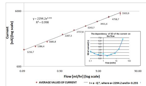
Fig. 2. Dependency of cell current on flow (log scale axis).
