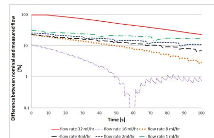
Fig. 4. Stabilization of the flow when flow is decreased to a half. The flow is expressed as percentage of nominal flow 1 – 32 mL/hr.
