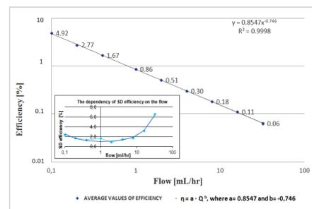
Fig. 5. Efficiency at different flow rates (log scale axis).
