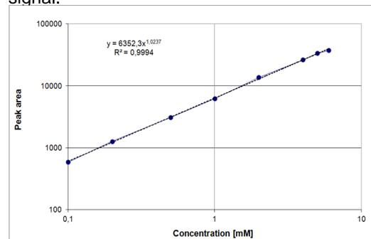
Fig. 1. Typical glucose calibration curve (dependence of current on concentrations).
