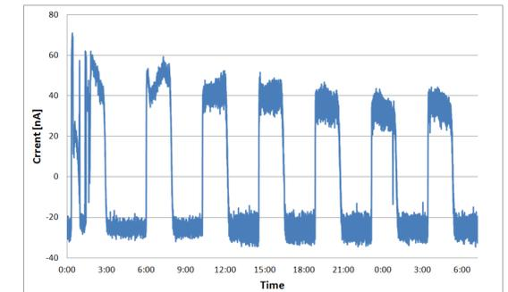
Fig. 4. The measurement of long-term stability GOD sensor with 3mM glucose solution.
