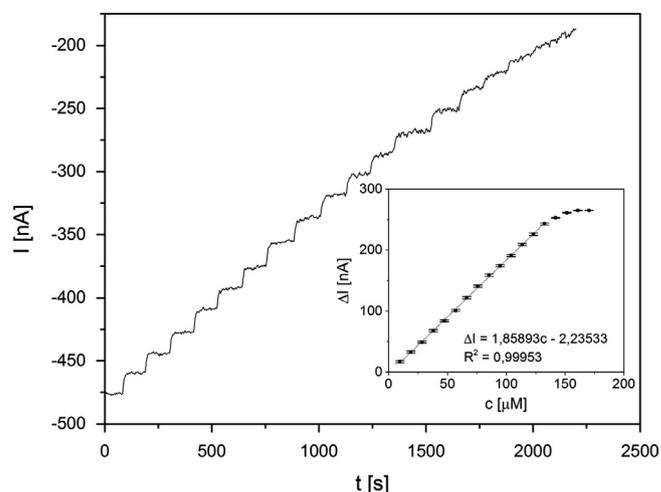
**Fig. 1.** CPMO biosensor signal as a function of CBCH concentration within the reaction chamber. Measured in phosphate buffer 50 mM, glucose 4 g dm<sup>-3</sup>, pH=7.0. Inset: calibration curve of CPMO biosensor processed by the least squares method.  $n=3$ , error bars shown in the graph.
