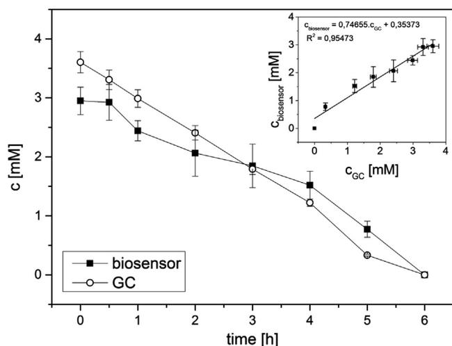
**Fig. 2.** Real samples measurement. Concentration of substrate CBCH in real samples from biotransformation measured by CPMO biosensor and GC. Inset: Correlation between biosensor and GC measurements of real samples processed by the least squares method.  $n=3$ , error bars shown in the graph.
